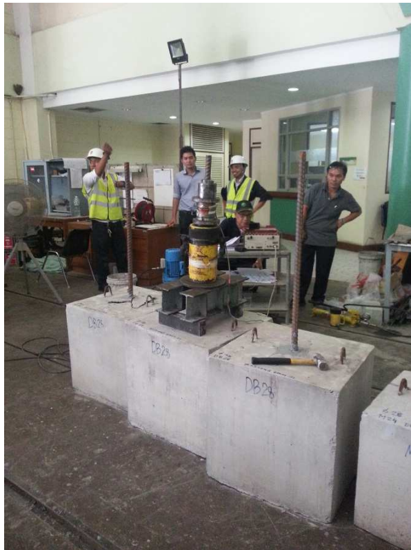
Non-confined test set-up for the pull-out test
